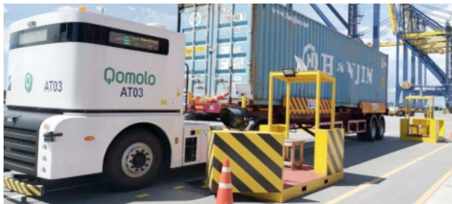
Centralised twistlock stations to protect stevedores handling twistlock cones
